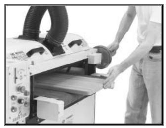
**Figure 49. ALWAYS** stand out of the way of where the workpiece could be projected, and keep fingers away from the underside of the workpiece.
